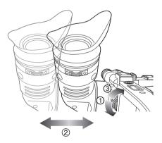
4 Adjust the diopter adjustment lever so that the characters on the viewfinder screen are seen most clearly.
